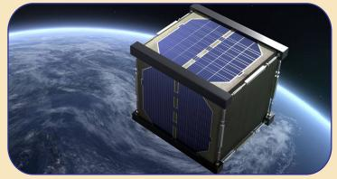
use any screws or adhesive materials, a joint effort by Kyoto University and Sumitomo Forestry Co., spending four years of arduous work at the project. Wooden satellites are seen as better for the environment when burning up upon reentering the Earth's atmosphere at the end of their operation, compared to conventional satellites made of metals, as they can create alumina particles, which may adversely affect weather and communications, according to the team.
